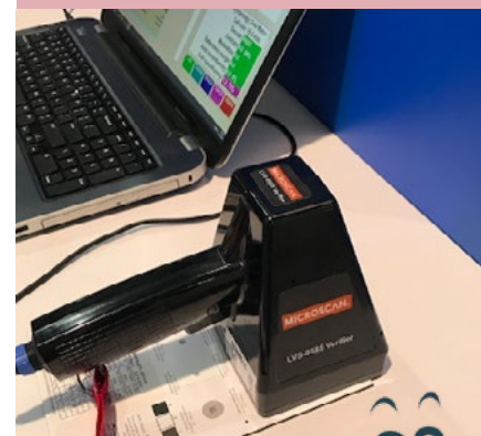
Below: A Microscan LVS bar code verifier analyzing quality
